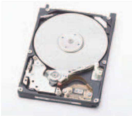
Robust storage solutions like the 2.5" HDD provide capacity to run vehicle infotainment systems
